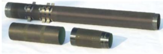
Figure 3: PAC-3 missile propulsion casing, a link piece and a radar casing, all made out of composite material [6]
