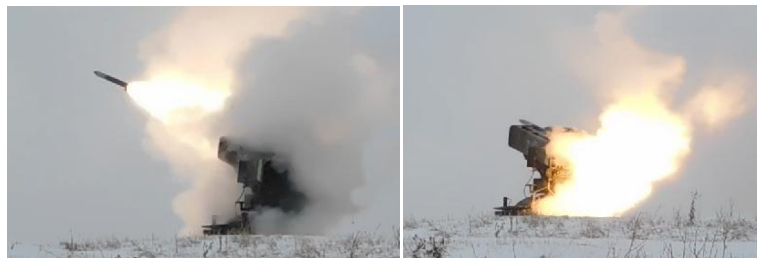
Figure 2 The gas jet generated by a 122 mm calibre unguided reactive projectile
