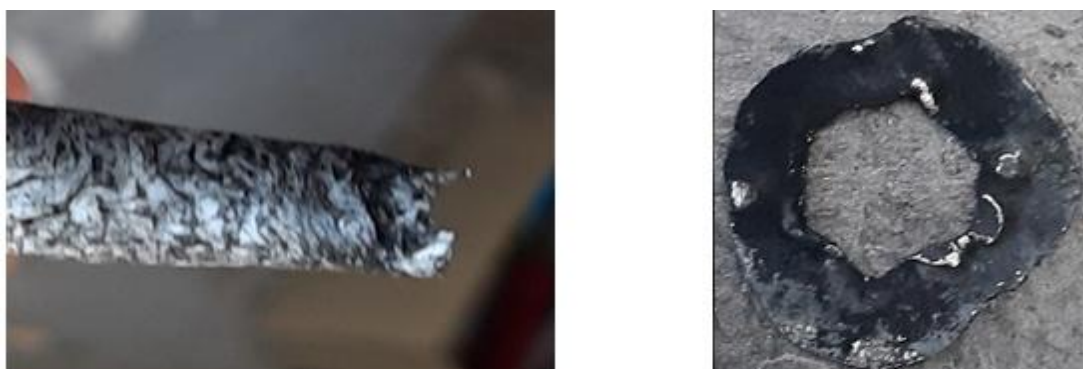
Figure 7: The piston in Teflon and the membrane in aluminum which reacted and took part in the combustion.
