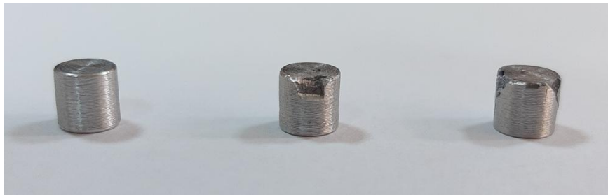
Fig.4 Samples aspect after the SHPB test
