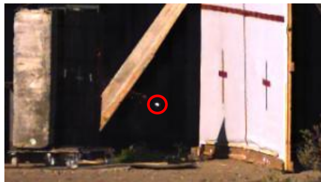
Figure 4: Bullet ricochet towards the panel
