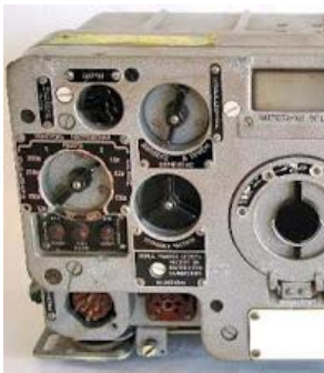
Figure no.1 R-123 radio station
